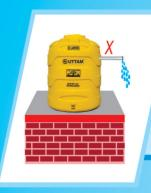
To utilise the complete capacity of the tank, DO NOT install the overflow pipe below the level of the inlet pipe.
