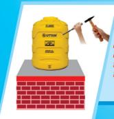
DO NOT use a chisel for making a hole on the tank for pipe fitting. this can crack the tank wall.
